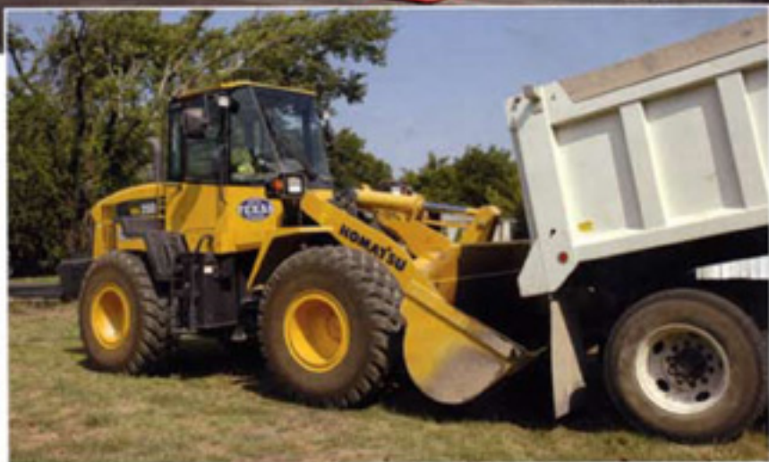
(Right) Mauricio Abrego with the city of Hillsboro takes on a load of asphalt mix with the Komatsu WA250-6 wheel loader, which he then uses to feed the city's asphalt paver (above).
